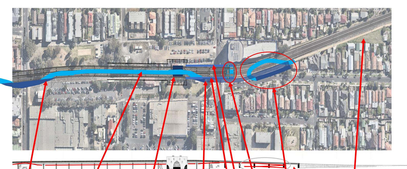
Veloway transition from Munro St bridge to under rail viaduct Veloway under Coburg Station Veloway access from station lifts below station level
