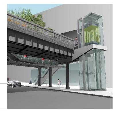
An illustration of a minimal ground footprint for an elevated railway station – e.g. north of Bell St and south of Moreland Rd. This concept design shows stairs in these locations.
